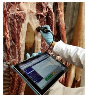
MN1700 miniature spectrometer analysing adipose tissue in pig carcasses in situ
